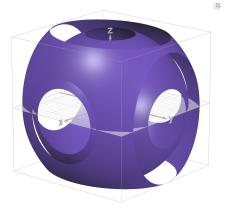
This equation can be solved for a particular frequency  $\omega$  to give the magnitude of the vector  $\vec{n}$  as a function of it's direction. This is a quadratic equation for  $n^2$  so in general there are two different magnitudes  $\vec{n}$  for a given direction. The function between  $\omega$  and  $\vec{k}$ .
